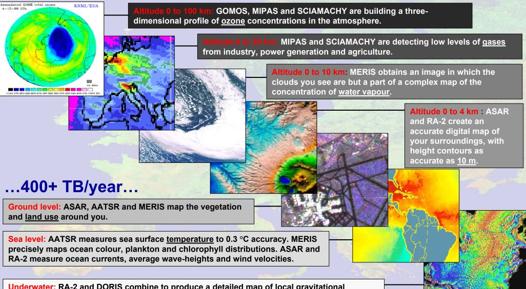
Underwater: RA-2 and DORIS combine to produce a detailed map of local <u>gravitational</u> strength, detecting the distribution of denser and less dense rock in the Earth crust beneath the oceans.
